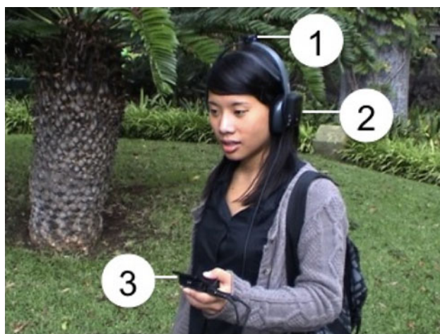
Fig. 1 Experimental setup. 1 JAKE sensor, 2 GPS receiver (both mounted on headphones), and 3 mobile device
