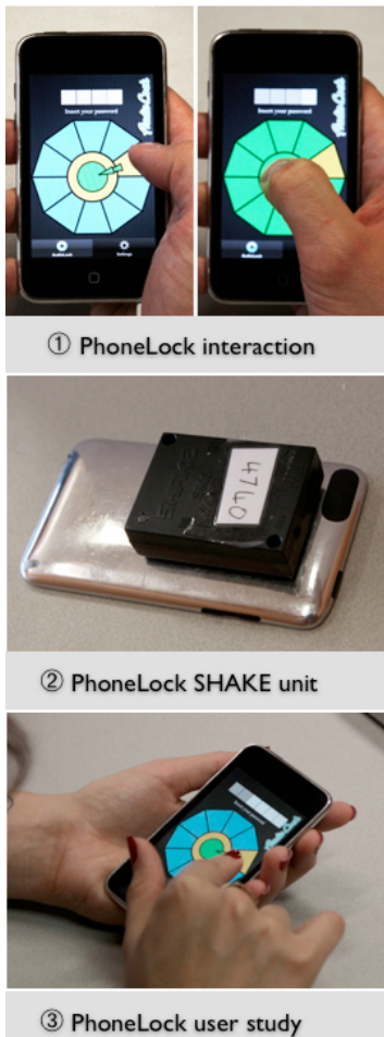
Figure 3. The PhoneLock system, the SHAKE unit attached to the back of the mobile device and a user test.
