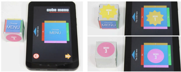
Figure 8: Command selection. Changing the orientation of a cube containing a magnet can be used to issue commands.
