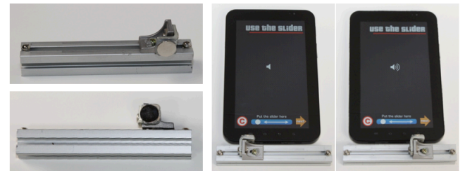
Figure 6: Linear movement. A magnet on a slider creates a linear one-dimensional volume control (center and right).
