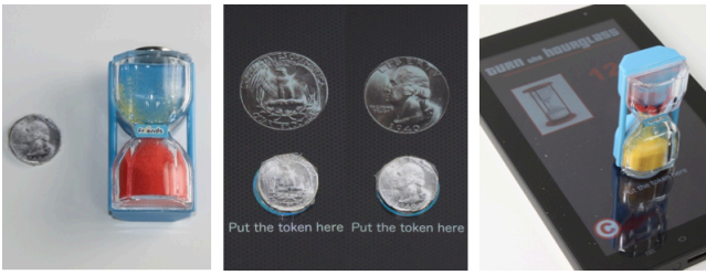
Figure 3: Flipping / orientation tokens. A coin and a hourglass afford detectable flipping actions (center and right).
