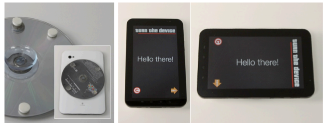
Figure 9: Device orientation. A magnetic turntable (left) allows the detection of device orientation (center and right).
