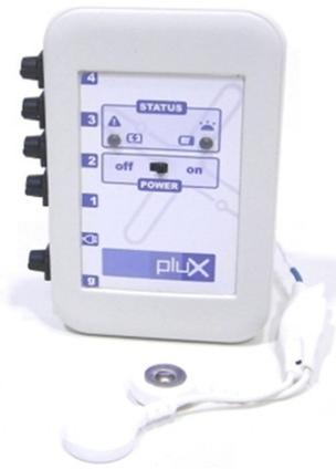
**Figure 1. bioPLUX biosignal acquisition device**
