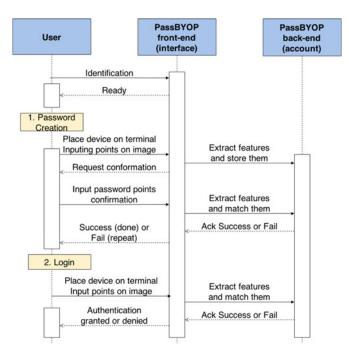
Fig. 1. Sequence diagram showing the steps involved in creating a PassBYOP password for the first time (1. Password Creation) and when attempting to login (2. Login).
