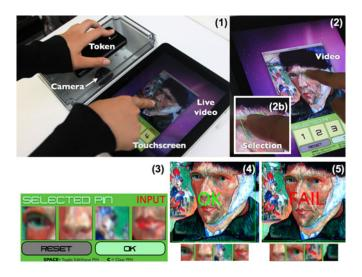
Fig. 2. (1) Overview of the PassBYOP system. (2) Input selection and closeup (2b). (3) Input selections that make up a password. (4) Successful authentication and (5) denied authentication.
