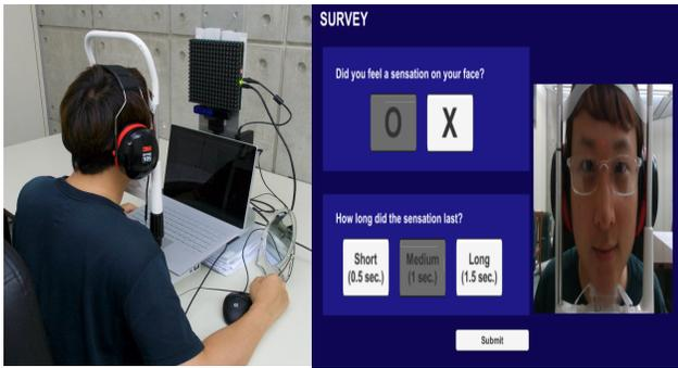
**Figure 1.** Left shows experimental setup including the UltraHaptics display and SR300 (depth camera) located 250mm in front of participants' faces. It also shows the laptop used enter data and answer questions. Right shows the experimental answer sheet for study 1. If participants answer 'O' to the first question, the second question and captured face figure appear. Cursor keys are used to move the red crosshair to the perceived stimulus location.
