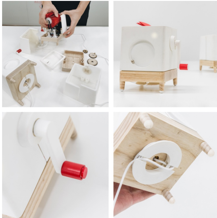
Figure 7. Rotation handle (bottom-left), inner mechanism for flipping top (top-left)
