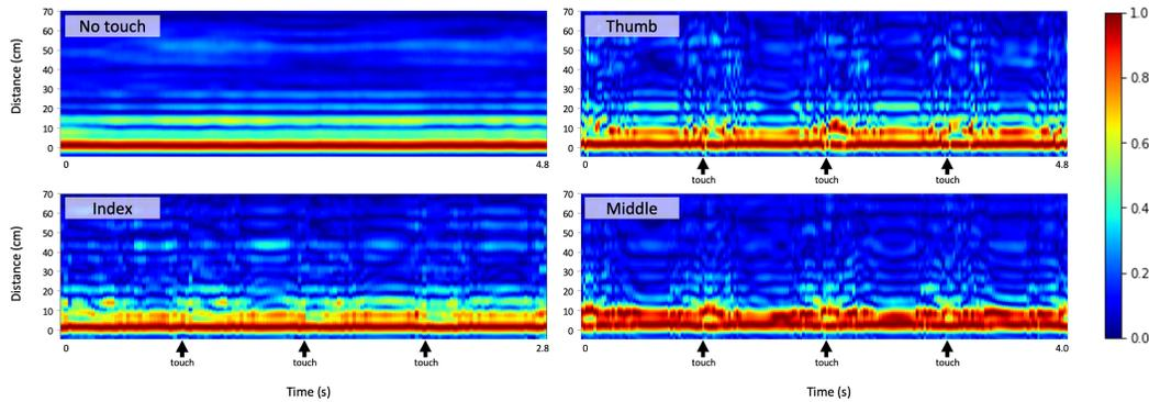
**Figure 2: Examples of the sonar fingerprints, or impulse response estimations, generated during periodic smartwatch taps by each finger. Top-left shows no tapping, top-right thumb taps, bottom-left index finger taps, and bottom-right middle finger taps. Finger touches are marked under the axes on each chart. In order to facilitate visual inspection, chart x-axes have different scales (to present taps at the same spatial interval) and y-axes show only half of the auto-correlated signal.**
