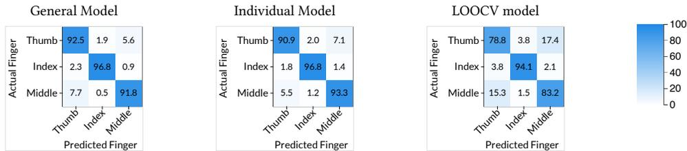
**Figure 5: Confusion matrices for SonarID classifiers (% accuracy). Left: general model; center: mean individual model; right: mean LOOCV model.**
