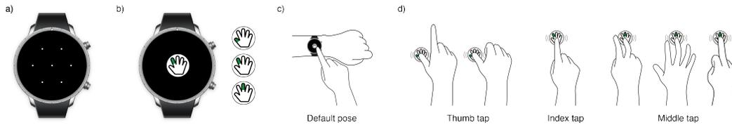
**Figure 3: Study interface and interaction. It shows target positions (a), the interface during a trial (b), the index finger pose used for taps to start a trial and during the fixation period (c), and representative examples of different participants' hand posture during thumb, index and middle finger taps (d)**
