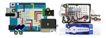
Figure 5: The Fritzing circuit used to power and control a servomotor using a potentiometer (left) and its physical layout in hardware (right). Letters show the components' mapping.
