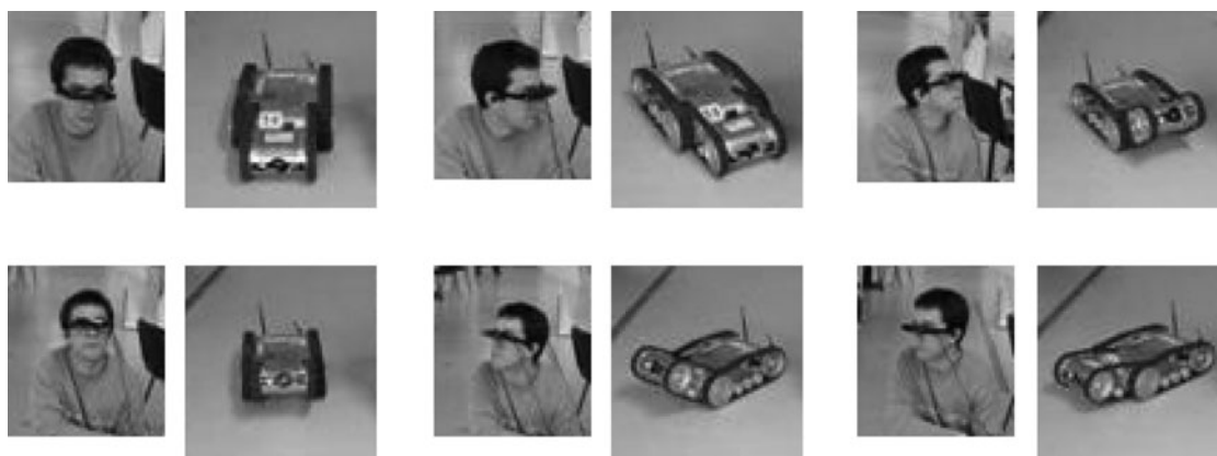
Fig. 5. Illustration of the HMD motion controlling the robot.
