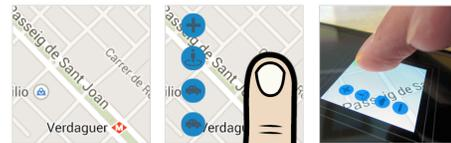
**Figure 9.** Demo map app (left). RL followed by L-Release shows a menu of options away from the right finger touching the screen (center and right). Subsequent taps with the raised left finger selects items.
