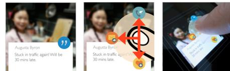
**Figure 10.** Demo message app (left). LR followed by L-Release shows a menu of options under the right finger touching the screen (center and right). Stroking towards icons and releasing, as in a pie menu, selects commands.
