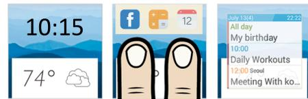
**Figure 8.** Demo home page (left). Dual-Tap brings up an app shortcut menu (center) and LR-Release, Dual-Release or RL-Release selects the left, center or right command respectively. In the example, RL-Release selects calendar.
