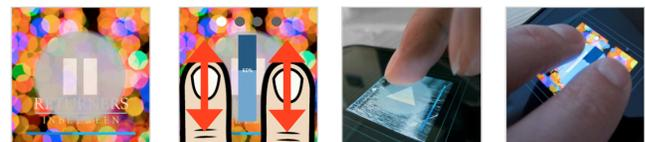
**Figure 12.** Demo music player (left). Single taps toggle play/pause while Dual-Tap shows a volume slider adjusted by vertical movements (left-center, right). After RL followed by L-Release, subsequent taps with the left finger goes to previous songs (right-center). LR followed by R-Release enables a similar interaction for subsequent songs.
