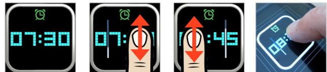
**Figure 11.** Demo alarm app (left). RL followed by L-Release triggers a slider and vertical strokes set hours (left-center, right). LR followed by R-Release sets minutes in a similar way (right-center). Dual-Tap followed by Dual-Release (not shown) toggles between clock & alarm modes.
