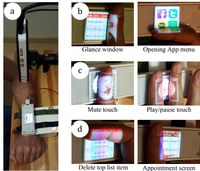
**Figure 7. Projector setup can be seen in (a). Image sections (b), (c) and (d) respectively show area-touches from the Watch Face Shortcuts, Media Player and Calendar Apps.**
