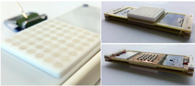
**Figure 3.** Left image shows close up of 33mm square sensor area standing 3mm proud of the surrounding surface. Darker circles are the touch sensor electrodes. Right two images show the device outside its casing from top (upper image) and bottom (lower image).
