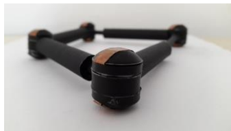
Figure 8: Appessory with connectors and copper tape
