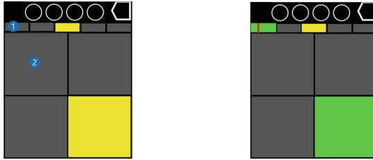
**Fig. 1.** GUI of PushID (left) showing touch force gauge (1) and buttons (2). Highlight items are in yellow. Example screen during input (right) showing red pressure cursor over first pressure level.
