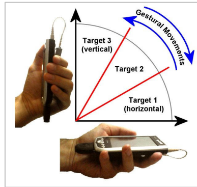
Figure 1. Illustration of the three target gestural input system. To use the system, the device is rotated between horizontal and vertical positions.
