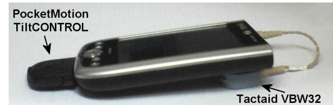
Figure 4. Hardware used to develop interface featuring motion sensor and vibrotactile display device.
